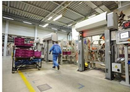
In orange, our safety roll up door RP300 with integrated safety limit switch PI e, cat.4
