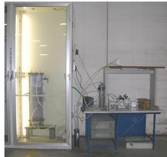
Anaerobic Membrane Bioreactor (Progetto Aquafit 4use)
