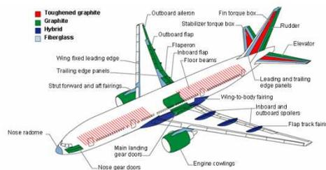
FIGURE 1-3 Production primary and secondary structure for the Boeing 777, an example of 1990s commercial application of composites.
