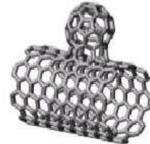
*Graphenated carbon nanotubes* by microwave plasma enhanced CVD
