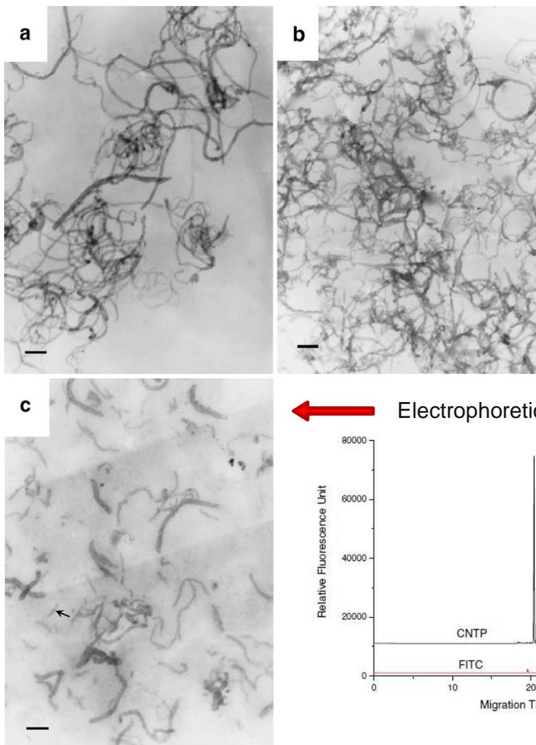
TEM images of multiwalled CNT before (a) and after (b) oxidation (COOH), and of fluorescently labeled CNTP (c). The scale bar corresponds to 200 nm. The arrow in (c) indicates a short oxidized multiwalled carbon nanotube
