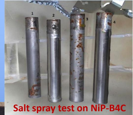
Salt spray test on NiP-B4C
