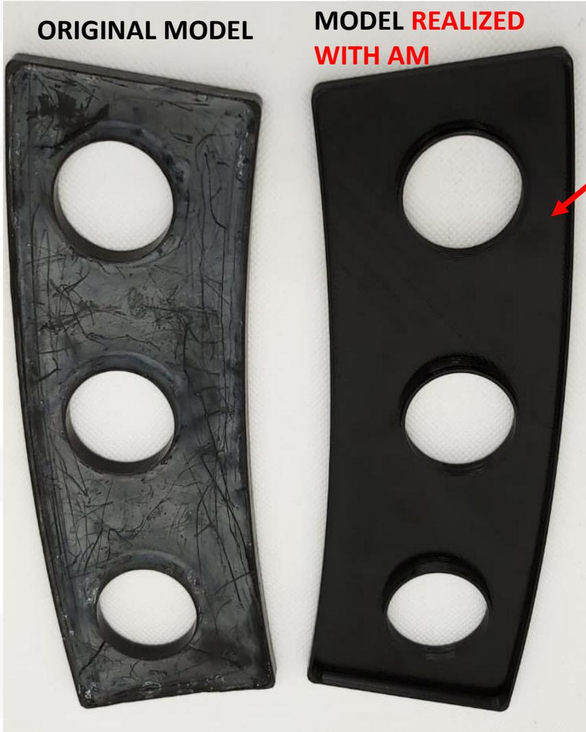
**Covering part for a CNC machine** in PC-ABS plastic:
