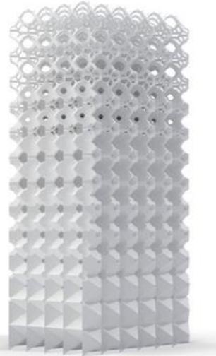
**Architected materials:** combinations of two or more materials, or one material and space (pores), designed to display attributes not offered by one material alone
