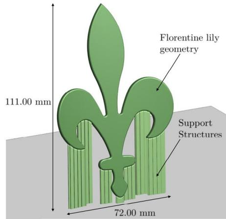
Original geometry and support structures
