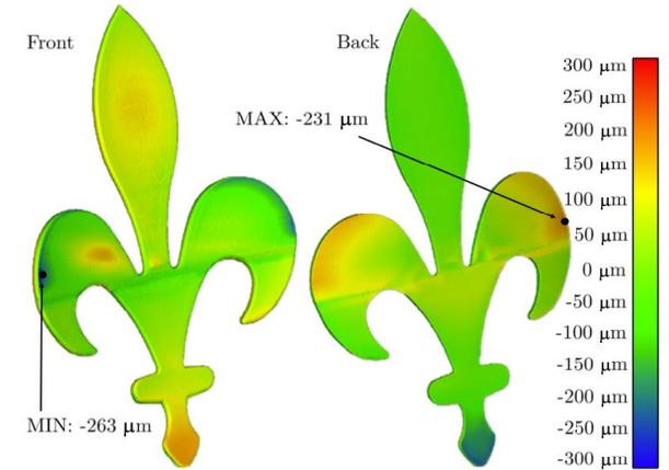
Relative displacements between numerical model and micro-CT
