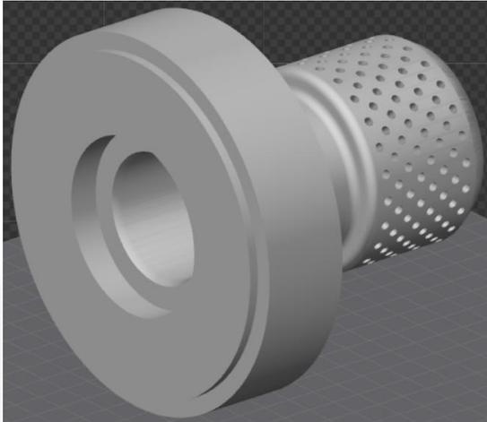
**AM component** in Stainless Steel: **50% of the original weight**
