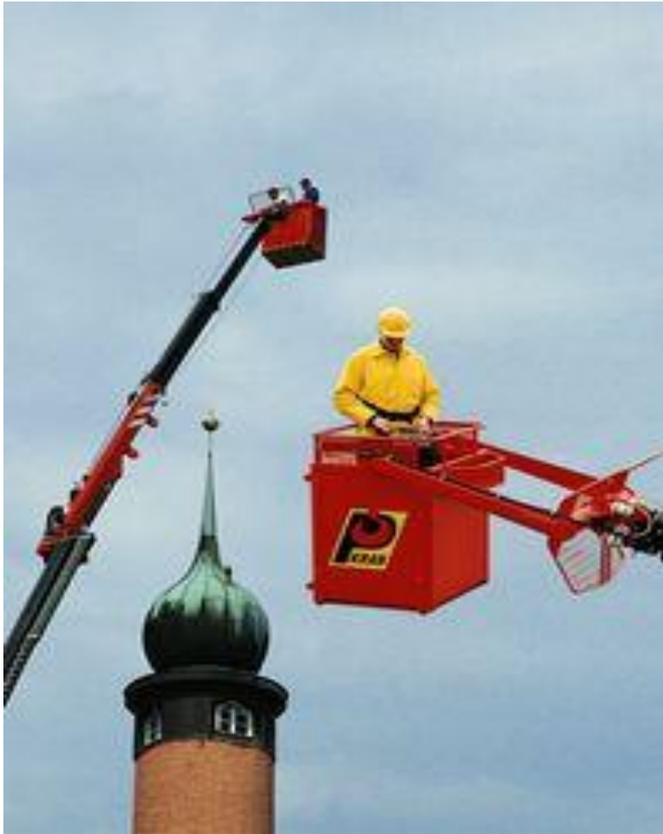
*Work platform assembled with a variable reach lift truck*
